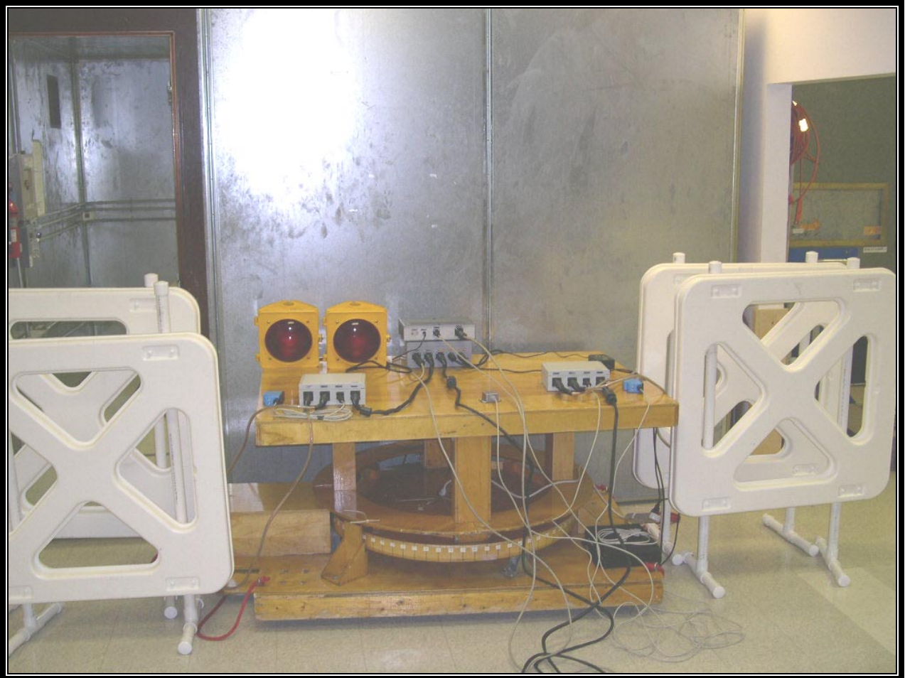
PHOTOGRAPH 1: TEST CONFIGURATION FOR DIGITAL RADIATED AND POWER LINE CONDUCTED EMISSIONS
