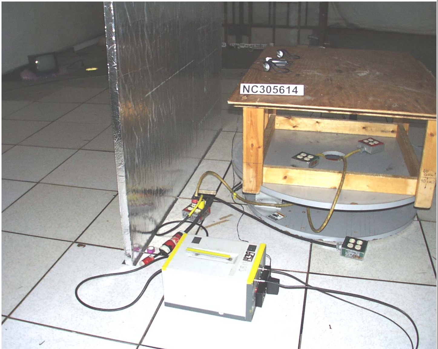
Test-setup photo(s): Conducted emission 10/150 kHz - 30 MHz
