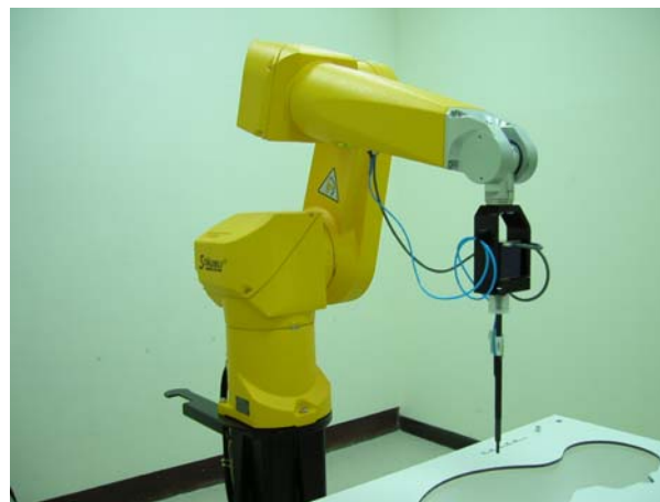
Fig. 5.2 Probe setup on robot
