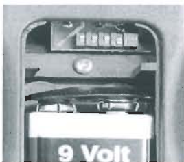
Figure 5: DIP Switch in Remote Handset Battery Compartment
