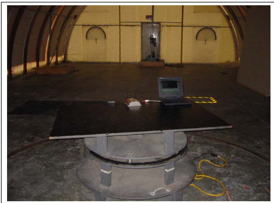
Figure 3.4-1 Radiated Emission Front View
