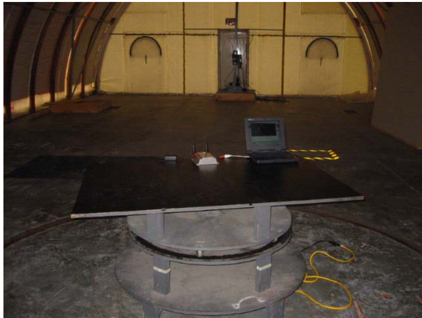
Radiated Spurious Test Setup, Front View
