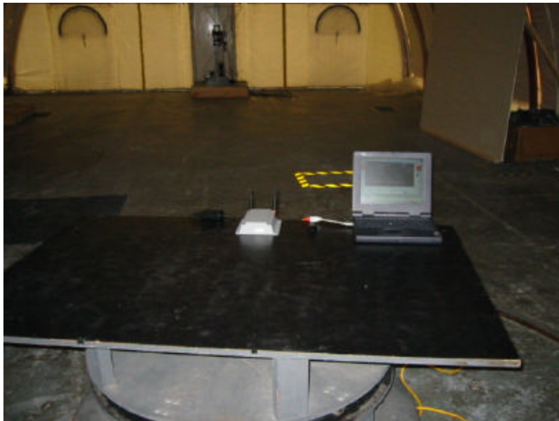
Radiated Spurious Test Setup, Front View
