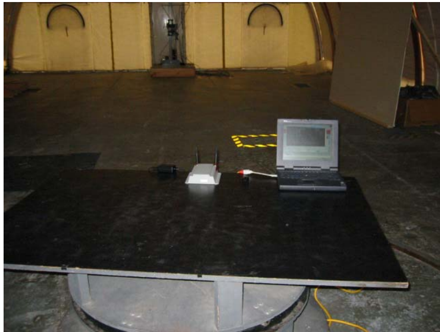
Radiated Spurious Test Setup, Front View
