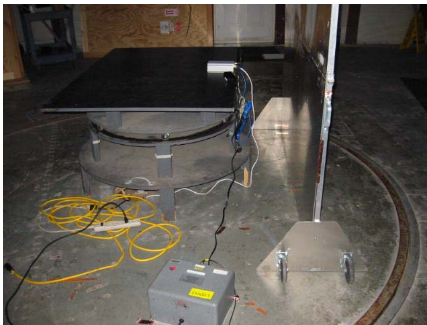
Power Supply Conducted Spurious Test Setup, Side View
