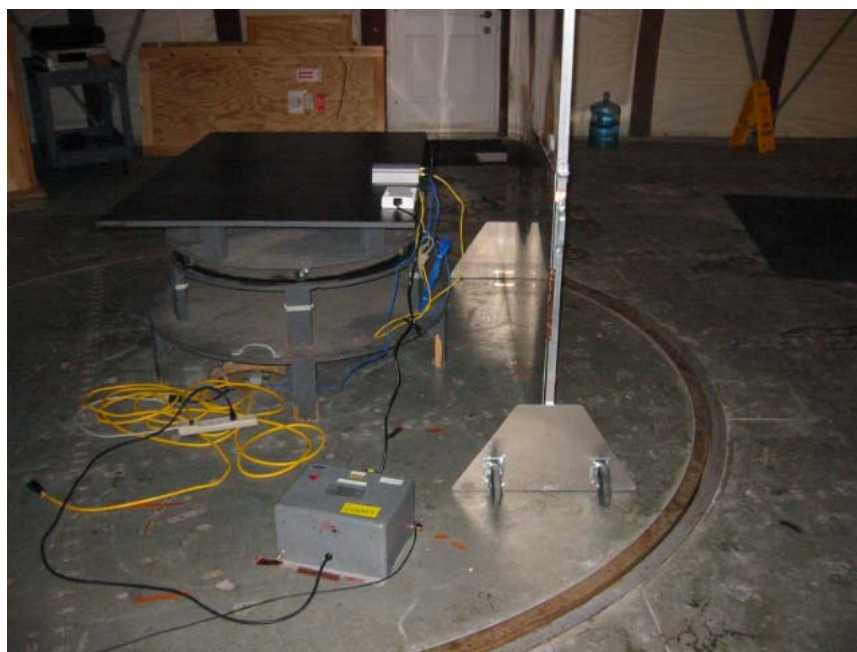
Power over Ethernet Conducted Spurious Test Setup, Side View
