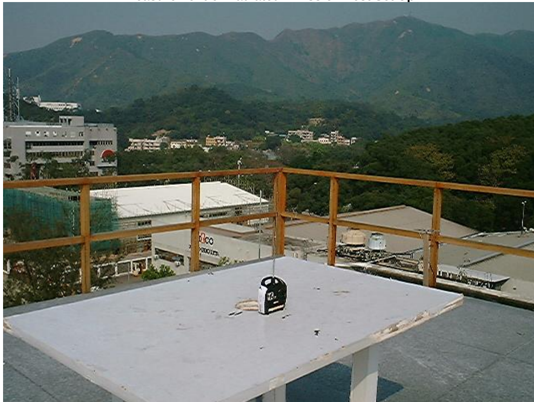
Measurement of Radiated Emission Test Set Up
