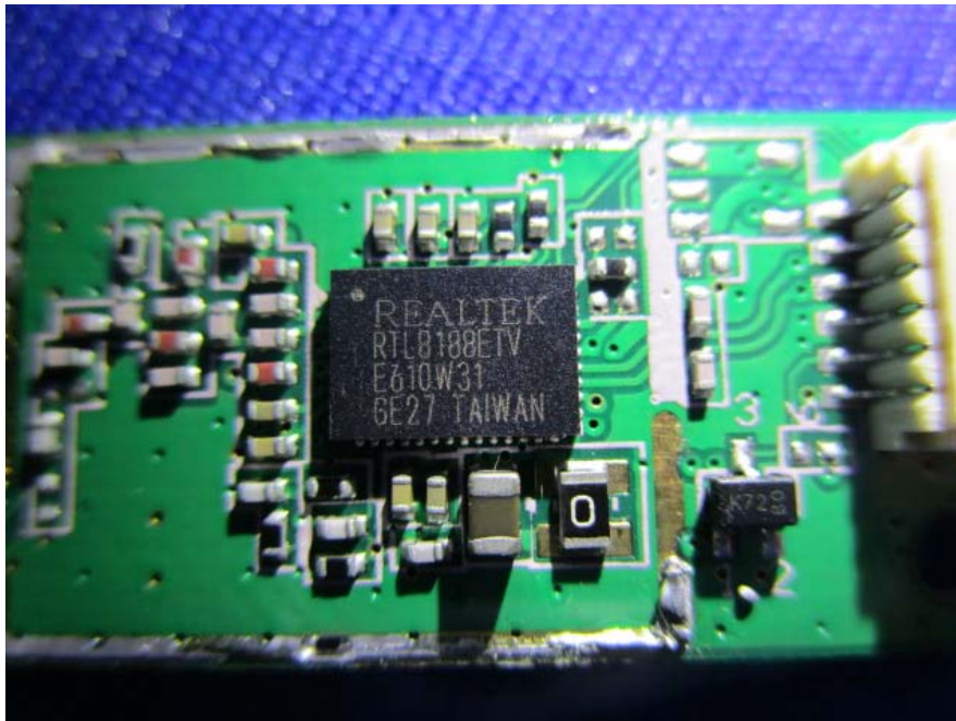
EUT –RF Chip View
