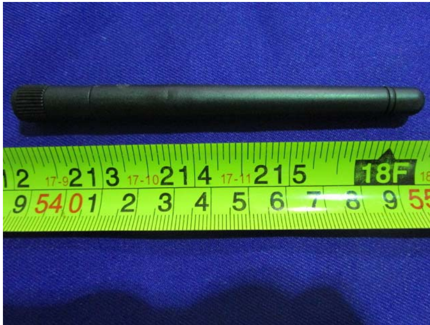
EUT –Antenna View (Skylink IWX-2411RSXX)
