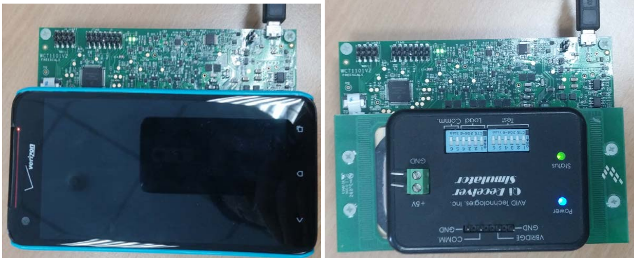
Figure-3 WCT-5WTXMULTI charging the equipments
