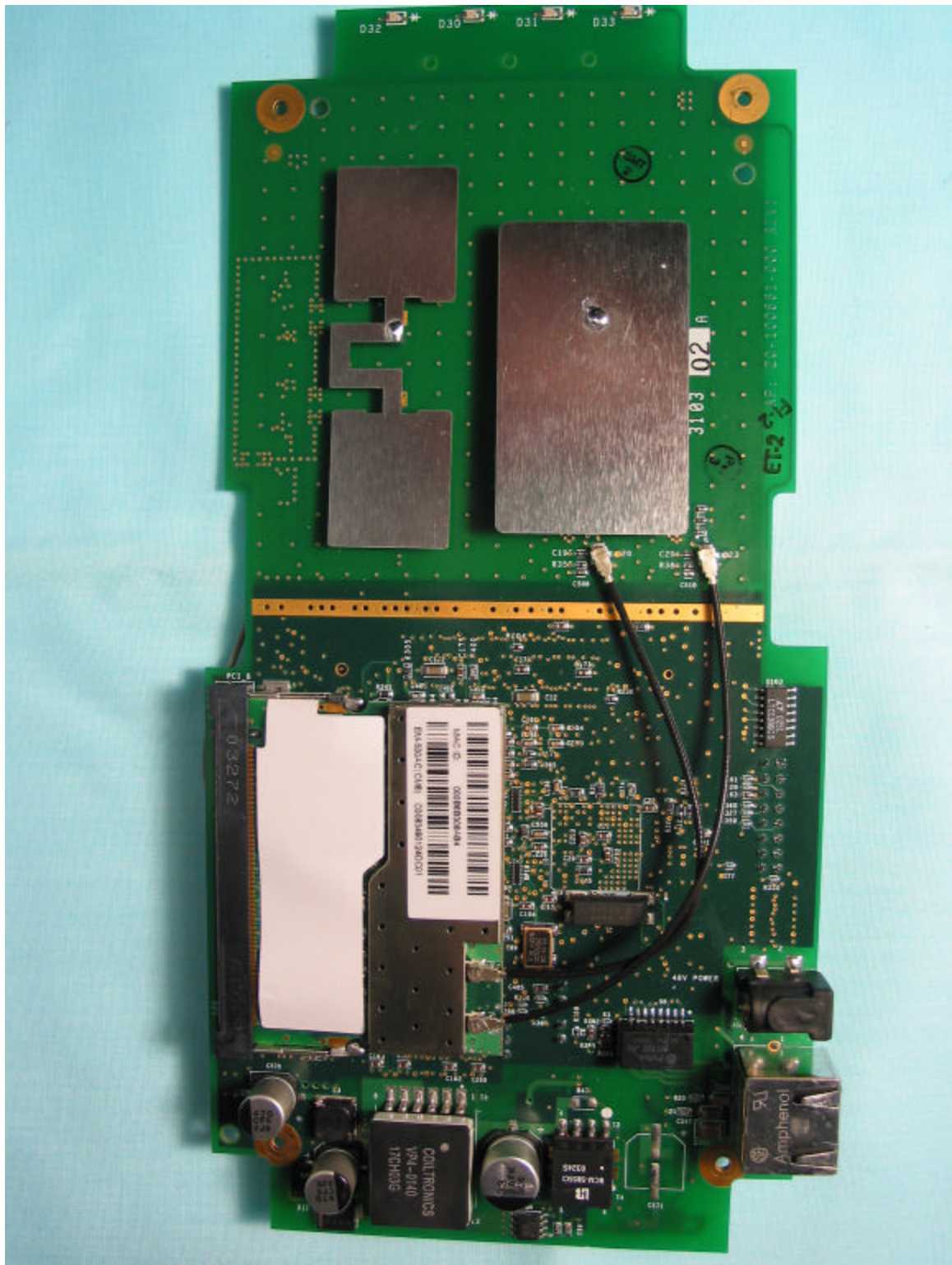
802.11 Access Point PCA, 802.11 BG side
