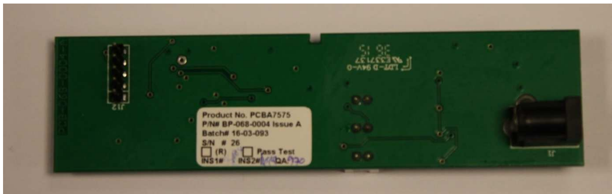
Case charger PCB – BP-068-0004 (Bottom)
