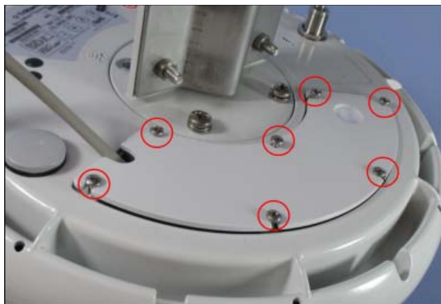
Figure 31 Cover for Ethernet connection
