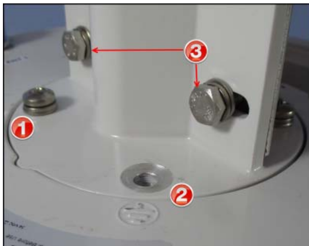
Figure 6 Clamp mount on Extender Bridge
