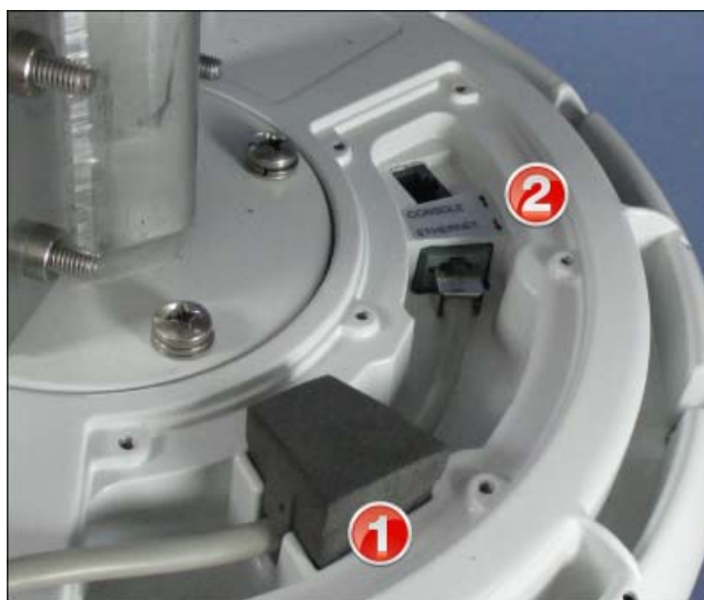
Figure 15 Ethernet cable for AL-0248 surge suppressor
