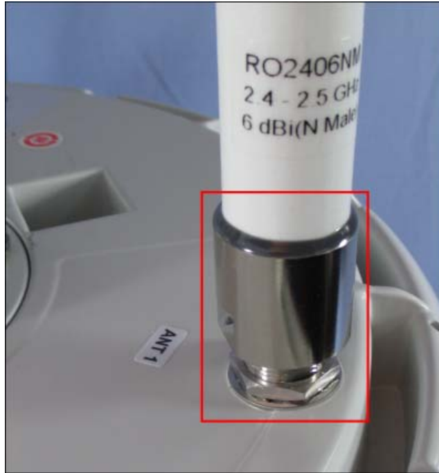
Figure 26 NAN Antenna mounted on base
