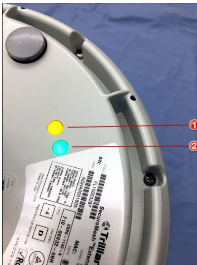
Figure 33 Link and Activity LEDs on base
