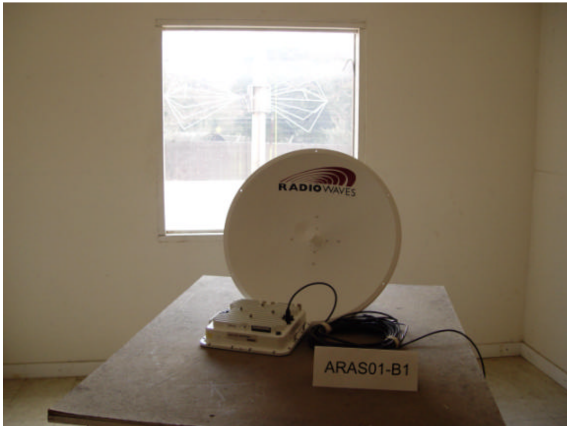
TEST SET UP 30M-1GHz Spurious Emissions
