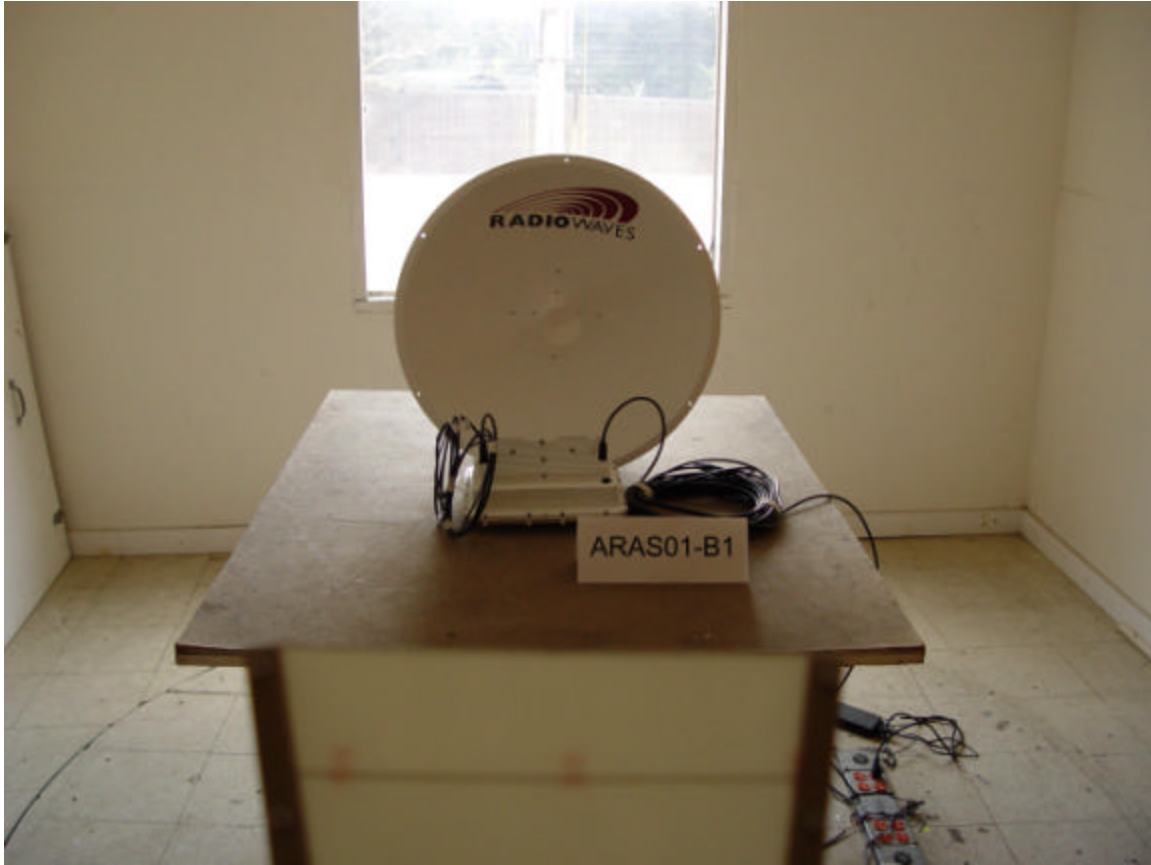
TEST SET UP 1-40GHz Spurious Emissions
