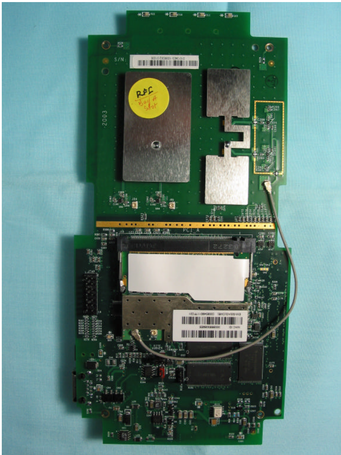
802.11 Access Point PCA, 802.11 A side
