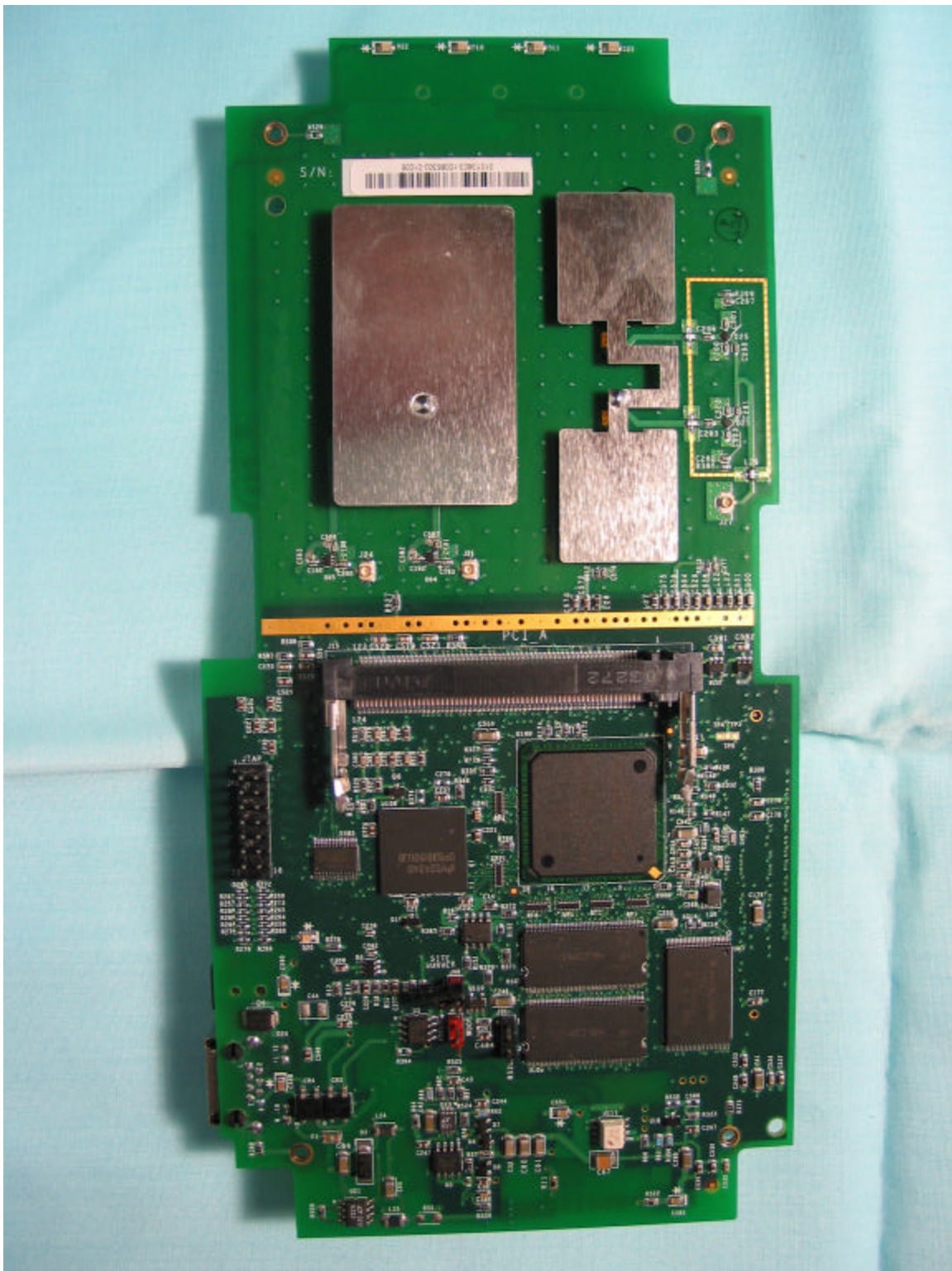
802.11 Access Point PCA, 802.11 A side
