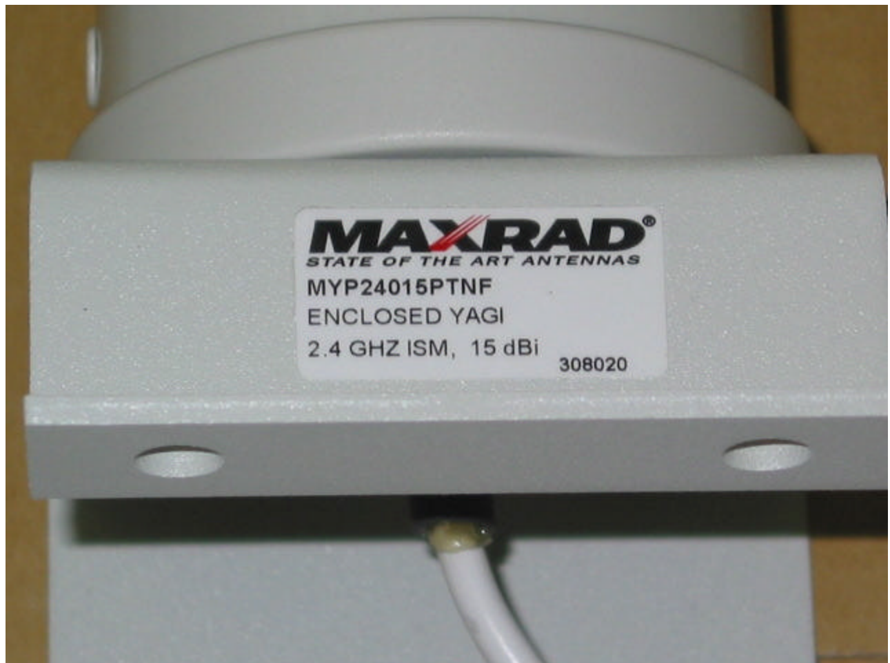
Radiated Emissions, 15 dBi Yagi, 2.4 GHz Antenna
