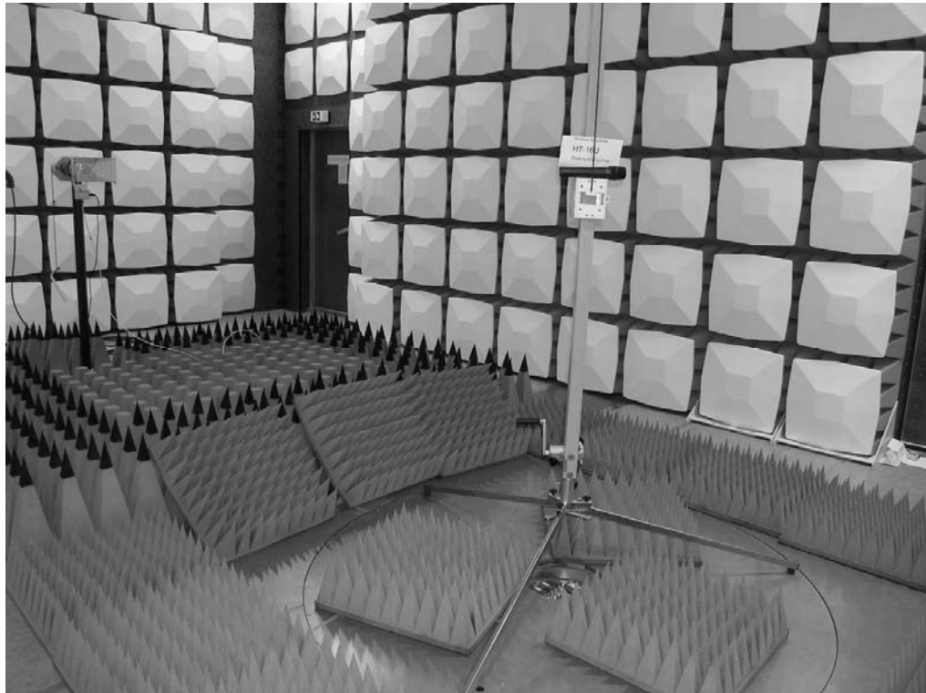
Photograph 2: Set-up for Radiation Measurement above 1GHz
