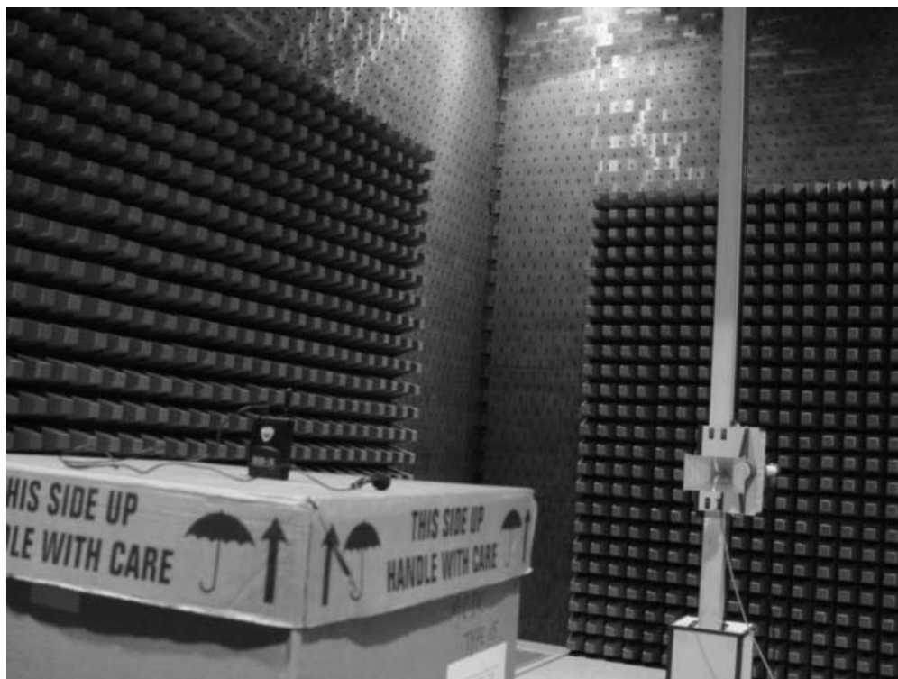
Photograph 2: Set-up for Radiation Measurement above 1GHz
