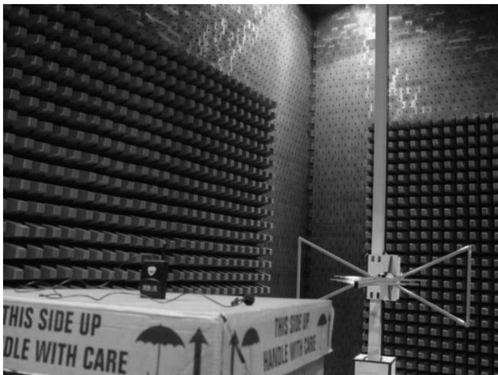
Photograph 1: Set-up for Radiation Measurement Below 1GHz
