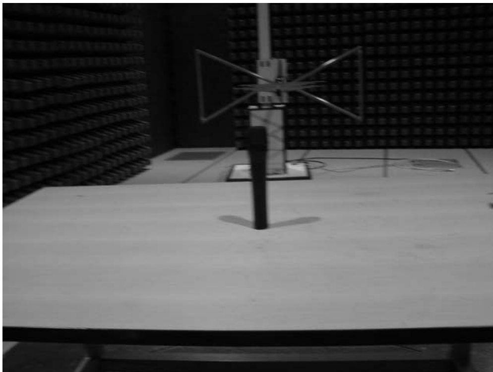
Photograph 1: Set-up for Radiation Measurement Below 1GHz
