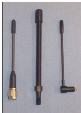
Full 1/4 models in straight and right angle
