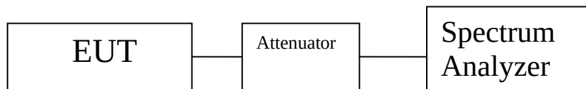
Figure 2. Block Diagram, Occupied Bandwidth Test Setup
