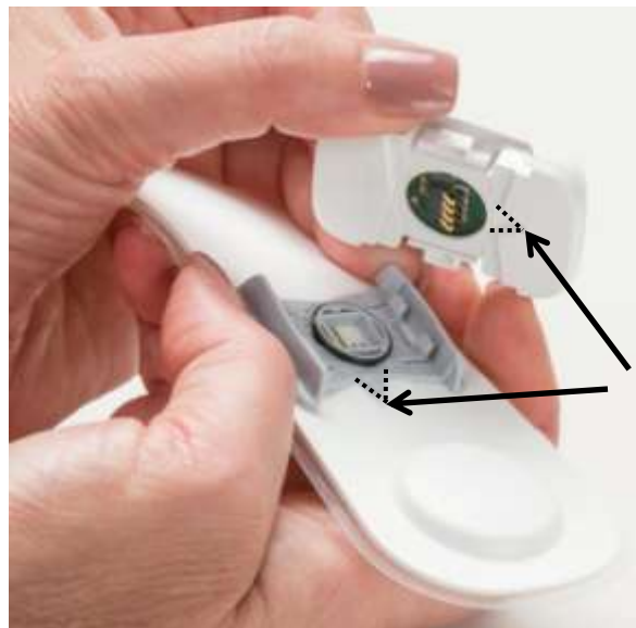
Figure 10: Align Triangles on Sensor and Patch
