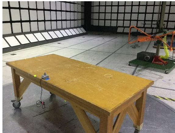
Figure 3 - Radiated Emissions Set up, Worst Case Orientation
