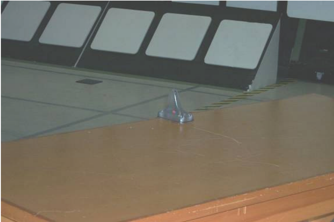
Figure 18 - Radiated Emissions Test Setup
