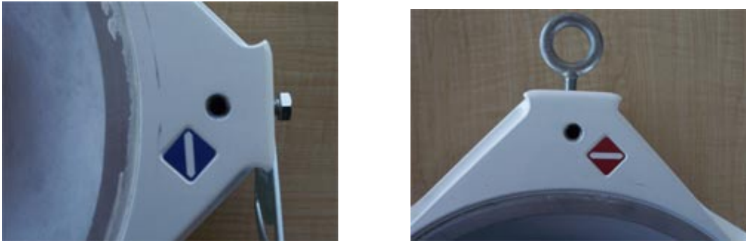
Figure 3-8.1: Polarization diamond orientations: horizontal (right) and vertical (left)
