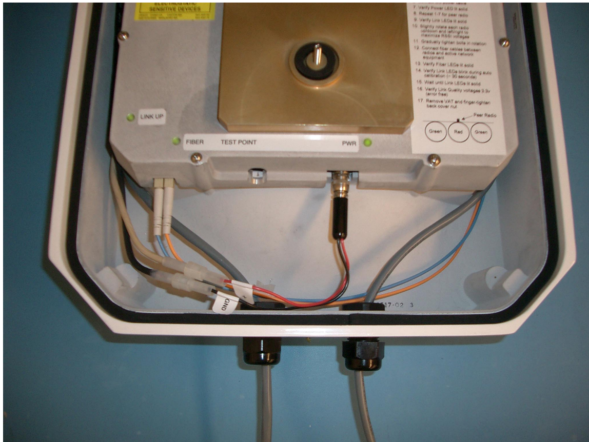
Figure 4-1: Link Up, Fiber and Pwr (Power) LED's indicating link is up and operating
