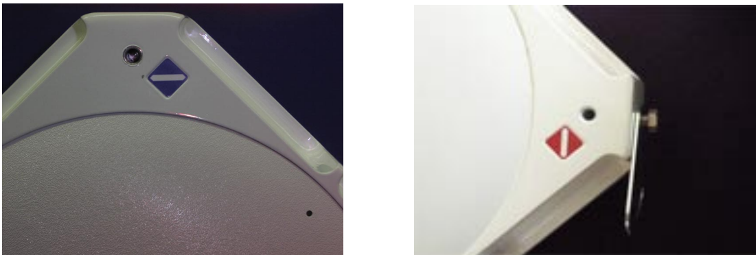
Figure 3-5: Polarization diamond orientations: horizontal (left) and vertical (right)
