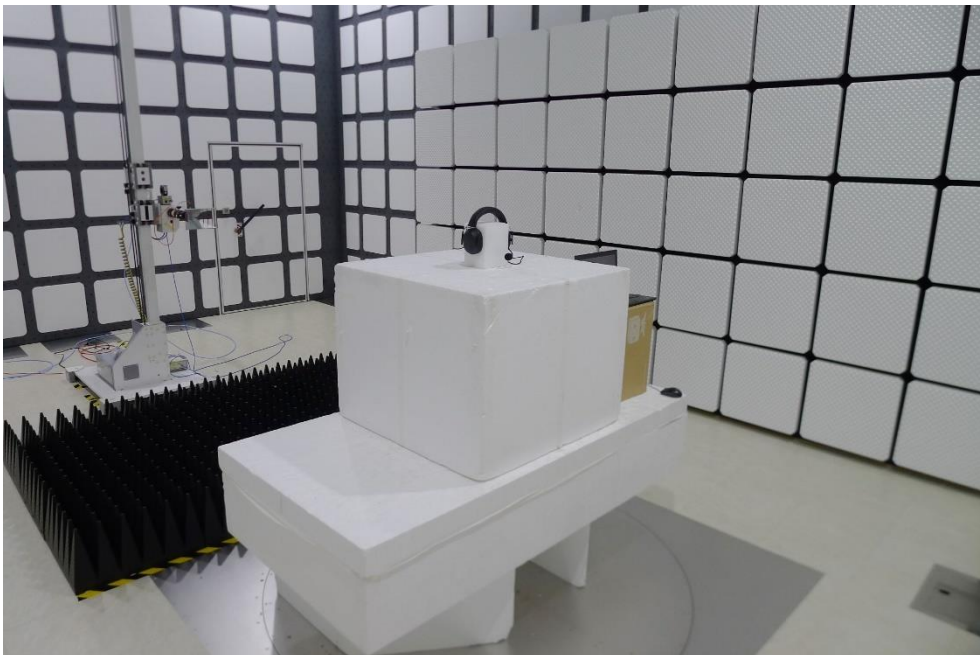
Description: Radiated Emission Test Setup for above 1GHz
