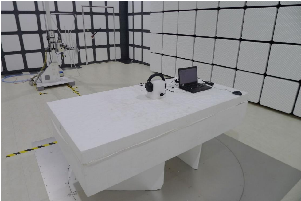
Description: Radiated Emission Test Setup for above 1GHz
