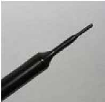
Figure 4.4 EX3DV4 E-field Probe
