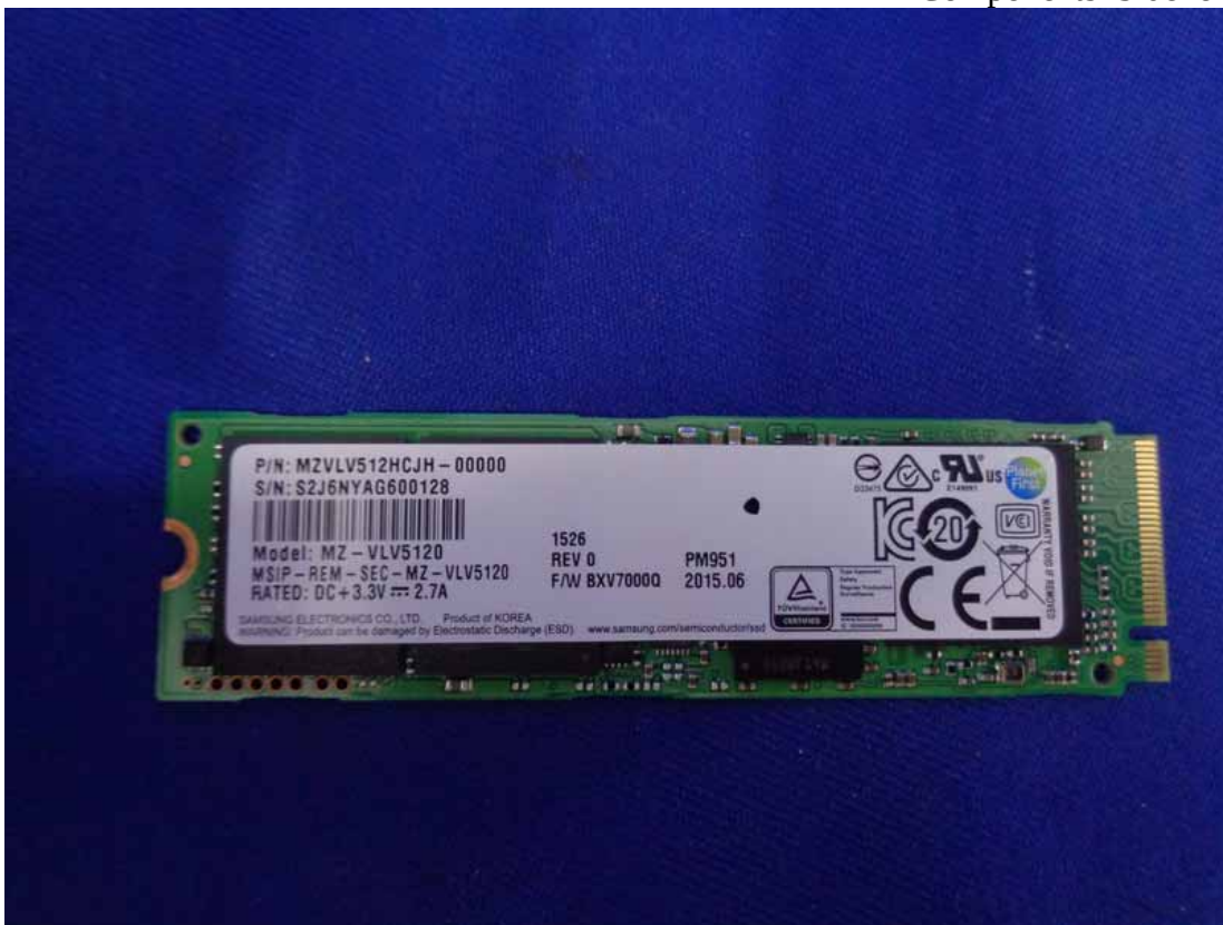
Figure 21 Components Side of the SSD
