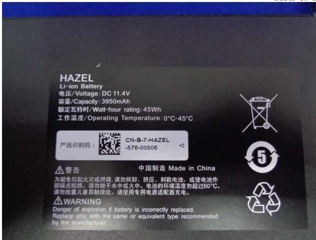
Figure 18 Label of the Battery
