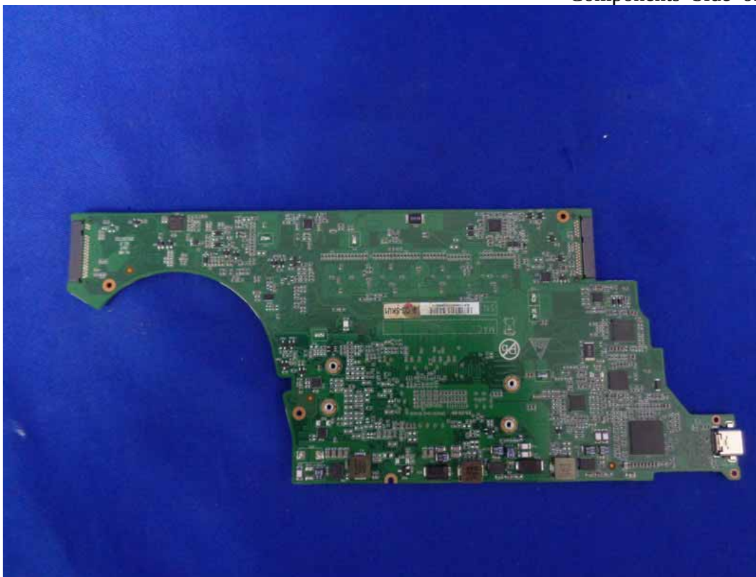
Figure 24 Components Side of the PCB
