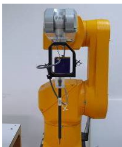
EX3DV4 E-field Probe
