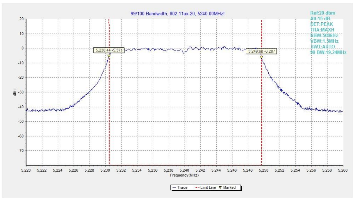
Fig.87 99% Occupied bandwidth (802.11ax-HE20, 5240MHz)
