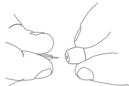
Use wire loop to clean wax from tips
