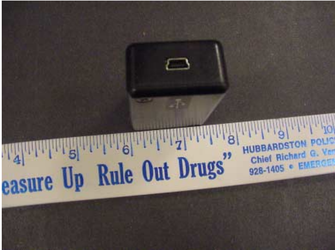
side view showing mini USB connector
