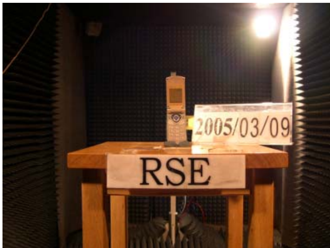
Pic2 Radiated Spurious Emission
