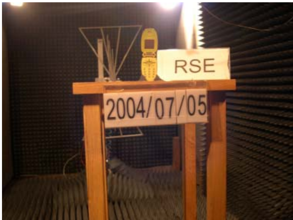
Pic2 Radiated Spurious Emission
