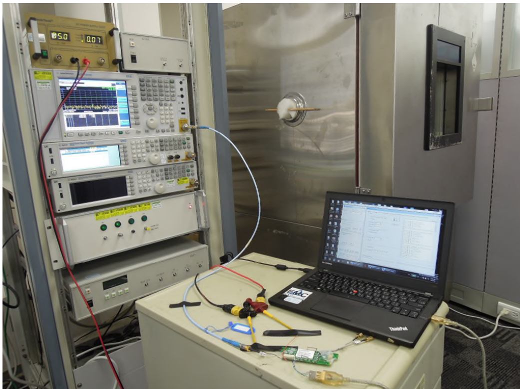
Photograph 4: Set-up for Conducted testing
