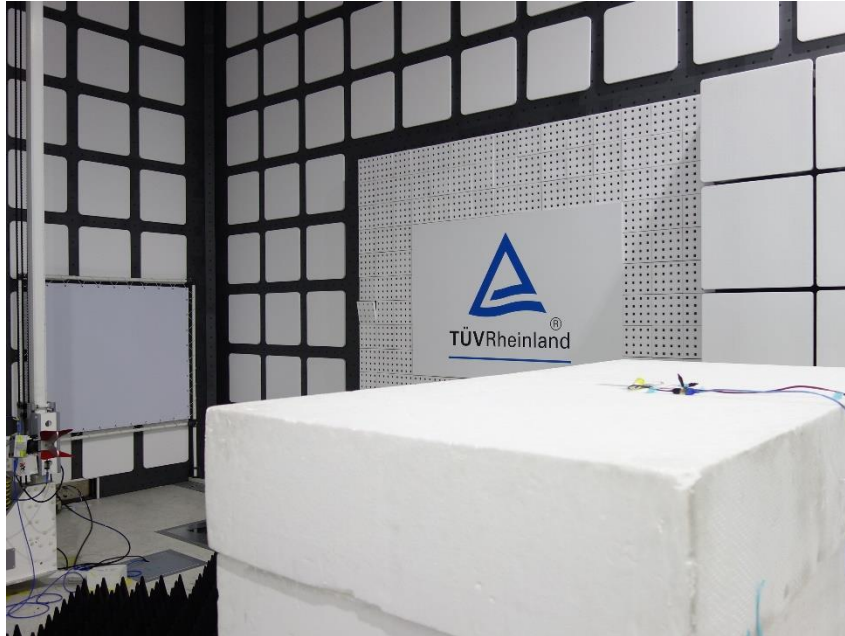
Photograph 5: Test Setup for Spurious Emissions (Back View 3)
