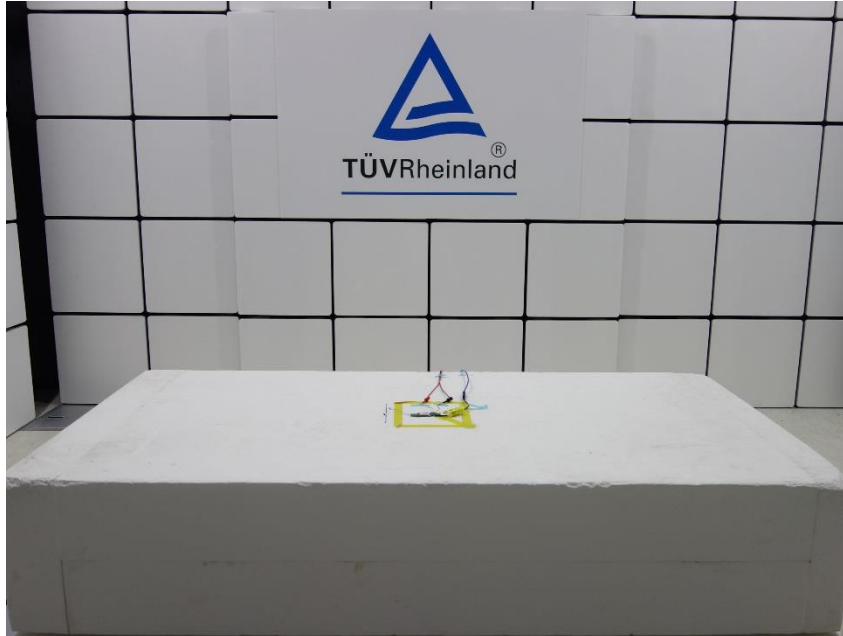
Photograph 1: Test Setup for Spurious Emissions (Front View 1)
