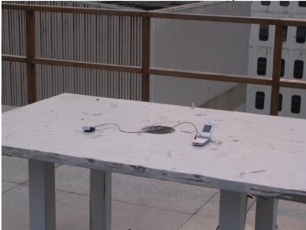
Measurement of Radiated Emission Test Set Up
