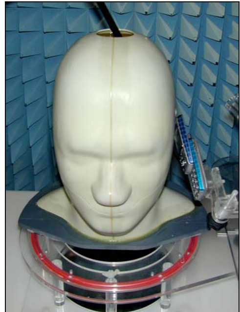
Figure 29. Positional photograph of MX-C99 Handset in the Left-hand 15 Degree Position
