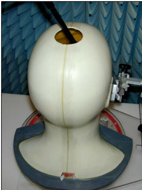
Figure 30. Positional photograph of MX-C99 Handset in the Right-hand Cheek Position
