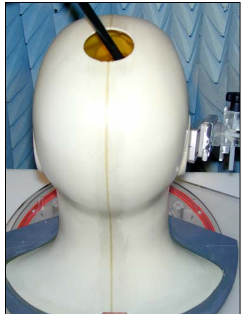
Figure 31. Positional photograph of MX-C99 Handset in the Right-hand 15 Degree Position
