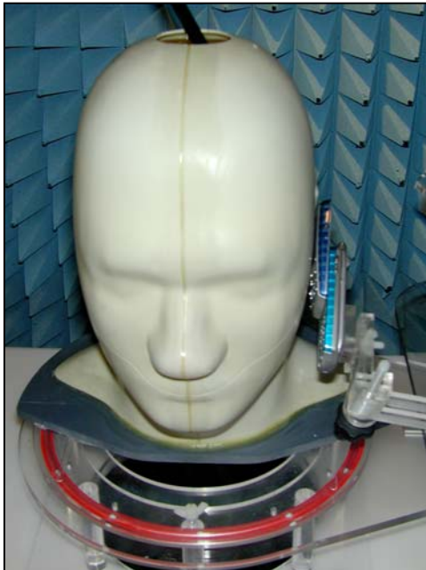
Figure 28. Positional photograph of the MX-C99 Handset in the Left-hand Cheek Position
