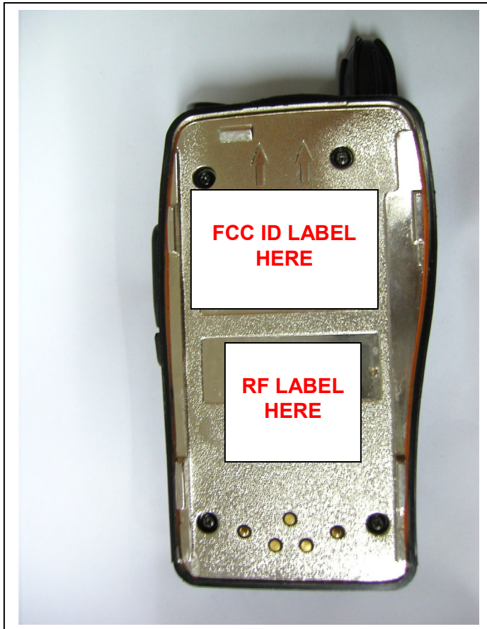
PHOTOGRAPH 1: FCC ID LABEL AND RF WARNING LABEL LOCATIONS
