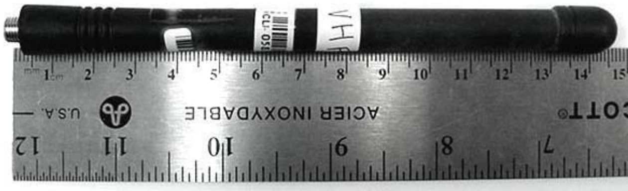
Whip Antenna (P/N: ACC-102)
