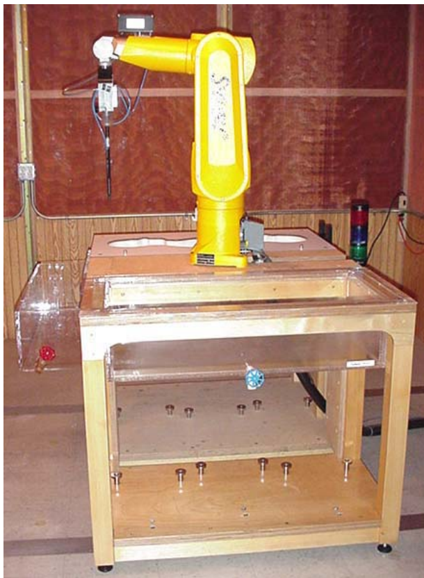
DASY4 SAR Measurement System with validation phantom
