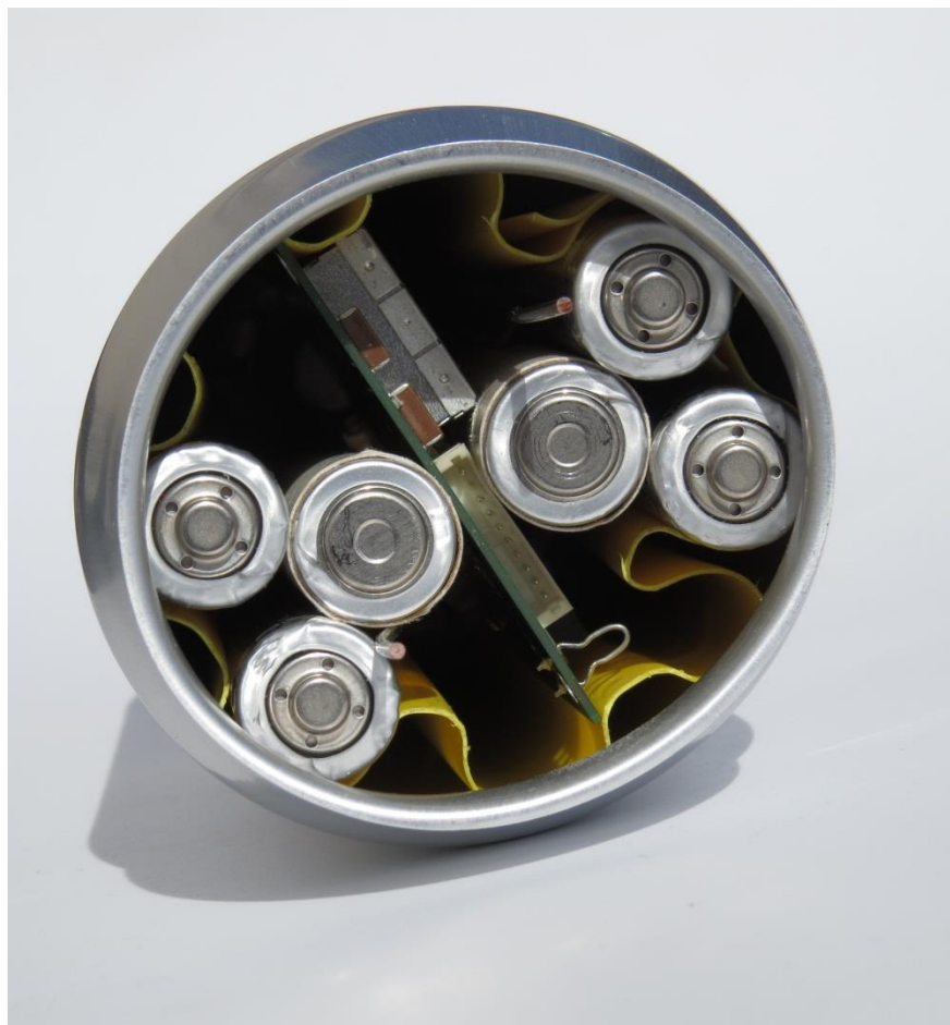
Radio Board with Batteries before lid seaming
