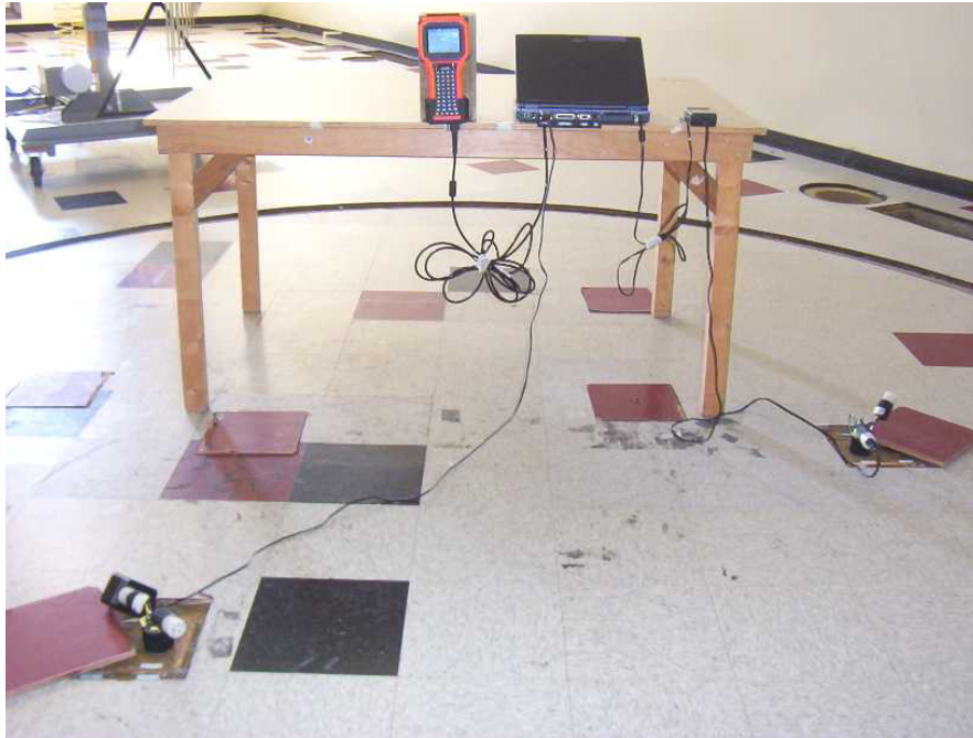
Photo 4: Radiated Emission Test Setup – Vertical Orientation, Front View
