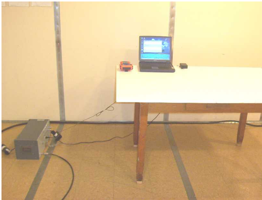
Photo 10: Conducted Emission Test Setup, JETT.XL – Front View
