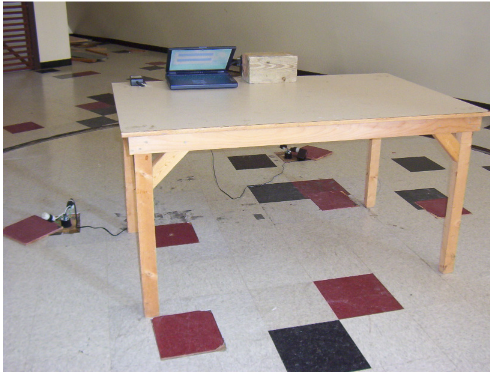
Photo 7: Radiated Emission Test Setup – Side Orientation, Rear View
