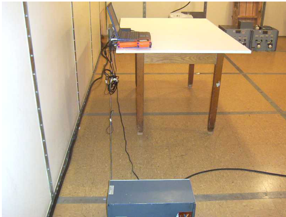
Photo 11: Conducted Emission Test Setup, JETT.XL – Side View
