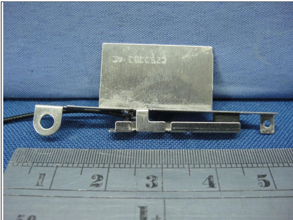
Antenna (Brand : WNC, Model : 81-EBJ15.005<3.62dBi>)
