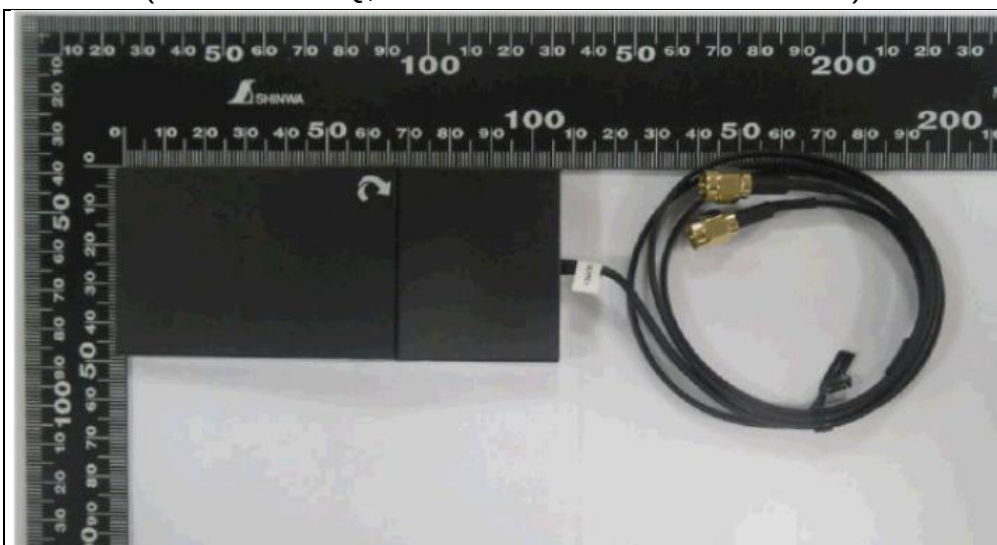
Antenna set 2 (Brand : INPAQ, Model : DAM-I6-H-DB-800-10-17)
