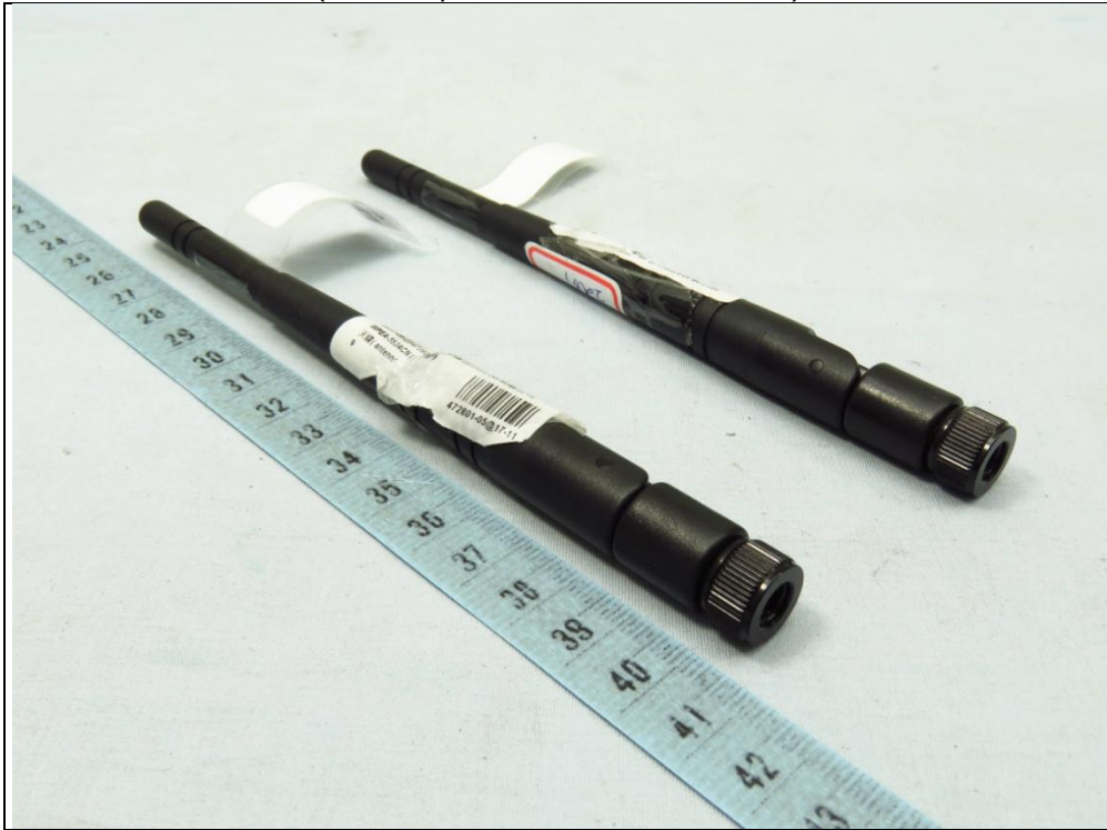
Antenna set 4 (Brand: Sparklan, Model: AD-103AG)
