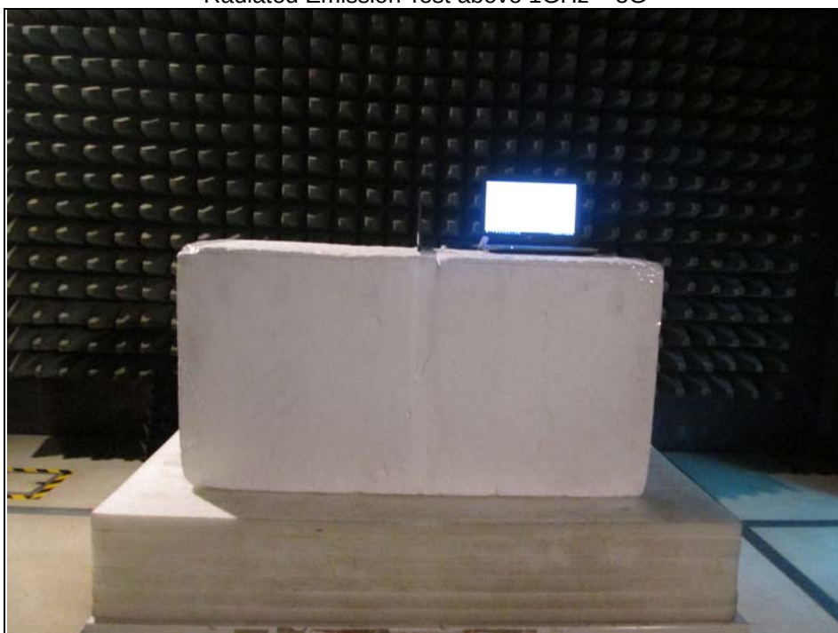
Radiated Emission Test above 1GHz – 5G
