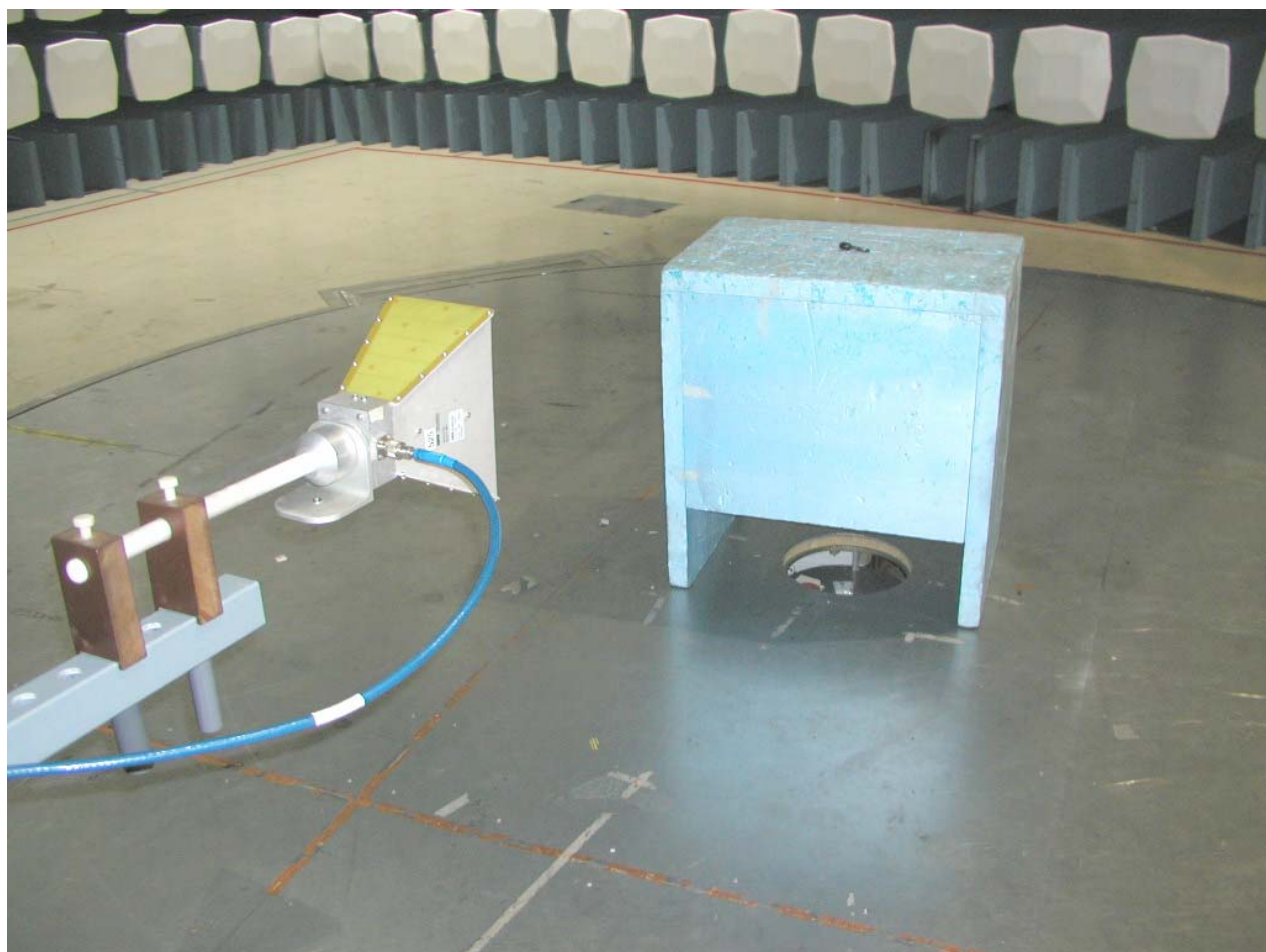
Photograph 2. Radiated emissions test setup
